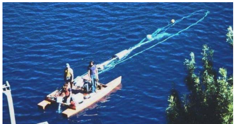
A Mackereth corer being prepared for deep-water sediment sampling operations in the Blue Lake in 1981 (courtesy Paul Harvey, 2008).
