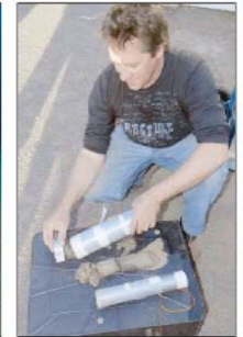
Deep dive team project manager Grant Pearce inspects sediment core samples taken from a depth of about 70 metres.
