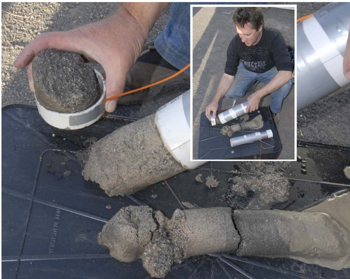
Some very unusual (presumably stromatolitic) formations found by the first trial dive team, and (below) Grant opening the first core tubes, revealing the first 30cm or so of layering of the Blue Lake's bottom sediments (RH).
