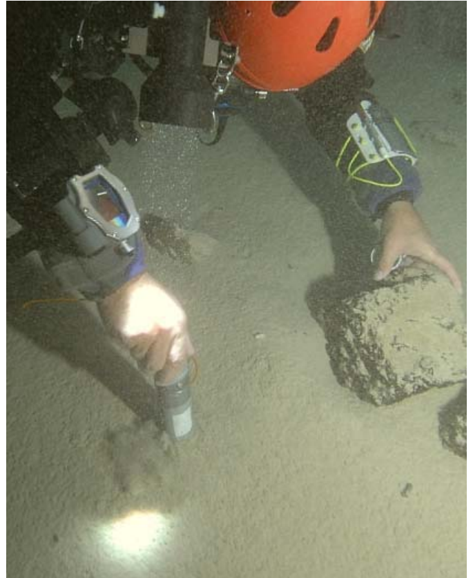
The first photographs of the silty bottom of the “bottomless” Blue Lake, taken by Richard Harris at a depth of 62 metres, served to verify the coring of the sediments out from the pumping pontoon. The short PVC coring tubes could easily be pushed into the soft powder-like silt.
